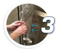
Start with a top outside corner and slowly peel a small section back. You can use plastic razor blades or a thin plastic putty knife to get under the film. Once you have a small section, stretch the film low to the paint and back towards the outside of the vehicle. When you stretch the film, it will release towards the inside with minimal stress on the paint.
