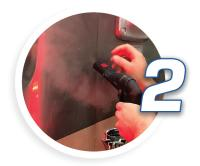
Paint protection film should be removed with a heat gun, wallpaper steamer, or infrared heat lamp. Only "warm" the film to reduce the risk of damaging the paint with too much heat.
