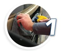
Depending on the condition and type of film, it can be helpful to apply a vinyl decal remover prior to peeling off the film. This will penetrate the top coat and help loosen the adhesive. Vinyl-off is an example of a good decal remover. Just apply on the film with a rag and be cautious not to get it on your headlights or fog lights. Applying two coats for optimal saturation is recommended. [www.crystaltek.us.com]
