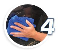
Once the film is removed there may be adhesive left on the paint. We recommend removing the adhesive using isopropyl alcohol or mineral spirits. Simply rub on with a rag. You can also try rapid remover by Rapid Tac (www.rapidtac.com) or "Adhesive Off" by Crystal Tek (www.crystaltek.us.com), just make sure to avoid contact with headlights as it will dull the plastic finish.
